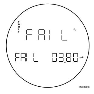
Figure 3-2. Faulted Operation Display
